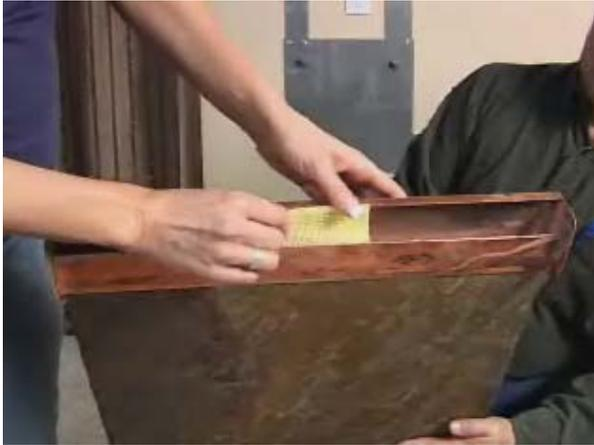
The next thing to notice is the baffling pad. The Water Distribution Unit should come with the pad already installed, if it is not or if you are replacing it, **(4) simply Bend the pad in half and insert it into the Water Distribution Unit in front of the water inlet nozzle.** In the area of the water inlet make certain the baffling pad slides all the way down and in front of the nozzle. Because the
