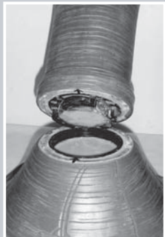
Screw the resin stand onto the resin base
